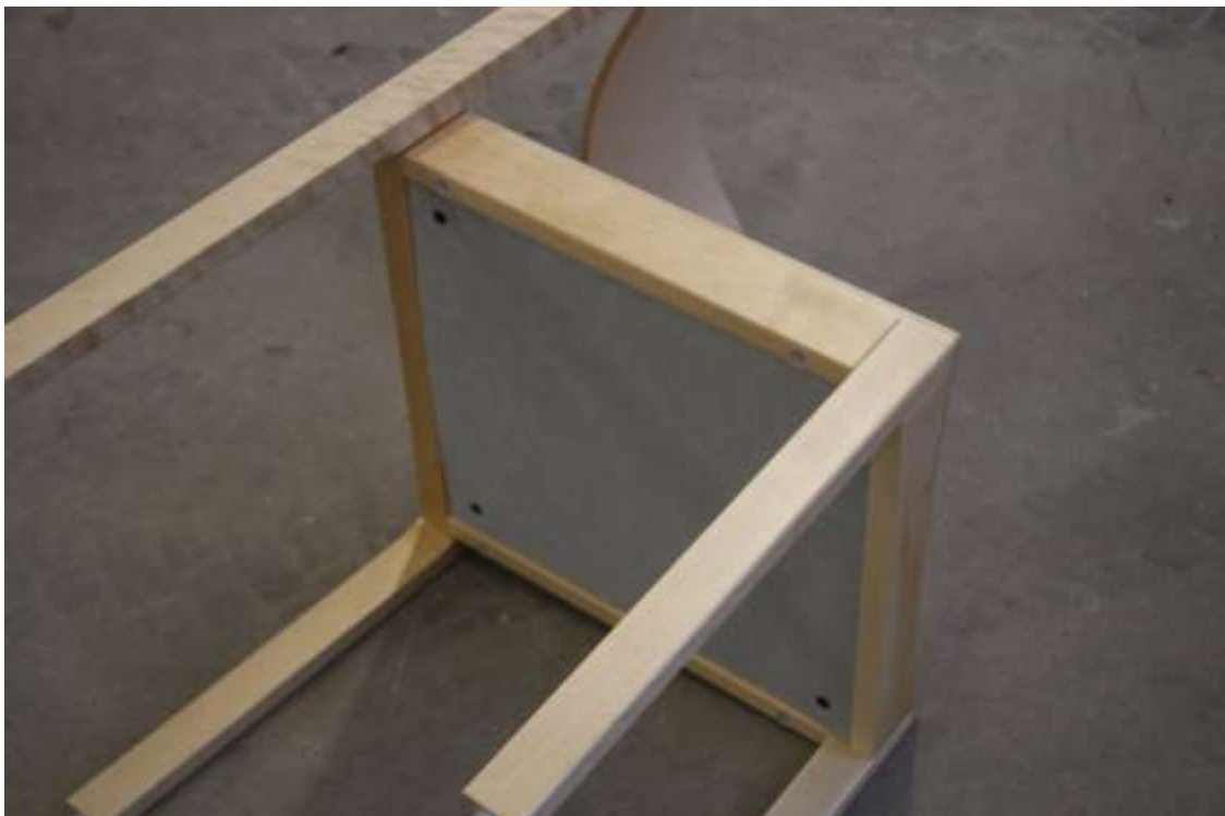
Picture 4 – One of the chairs with a sound absorbing pad on the underside.
